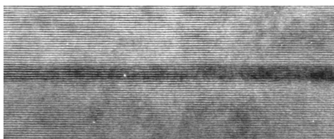
Figure 12. TEM image of a 3.5 nm thick \text{In}_{0.2}\text{Ga}_{0.8}\text{N}/\text{GaN} QW.
